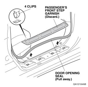
9. Pull away the door opening seal, and remove the passenger's kick panel.
