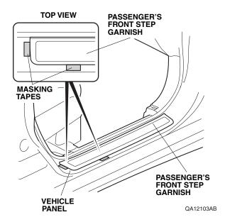
8. Pull away the door opening seal, and remove and discard the passenger's front step garnish.
