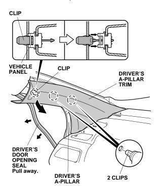
9. To prevent the clips from falling into the vehicle body, roll up the shop towel, and insert it between the driver's A-pillar and the dashboard. Take care not to damage the driver's A-pillar.
