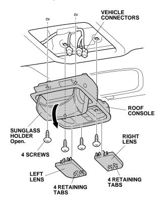
3. Remove the cover (two retaining tabs).
