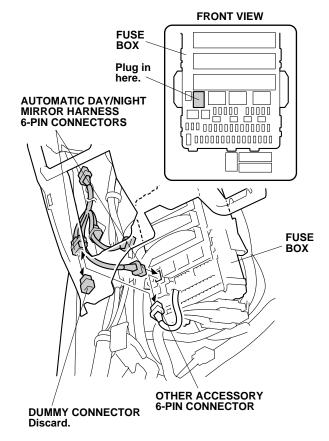
19. Remove the dummy connector from the automatic day/night mirror harness 6-pin connector, and plug the other accessory 6-pin connector to the automatic day/night mirror harness 6-pin connector.
