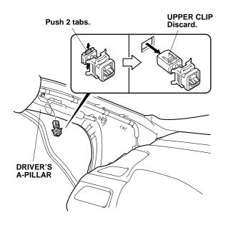
12. Remove the driver's dashboard panel (six clips and unplug the vehicle connector).
