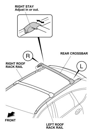
5. Secure the rear crossbar to the roof rack rails using four bolts. Torque the bolts to 10 N·m (7.3 lbf·ft).
