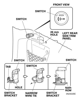
65. Align the tab on the switch bracket with the hole on the switch and secure the switch bracket to the switch with one narrow wire tie.
