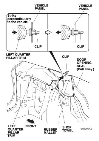
19. Using a rubber mallet wrapped with a shop towel, lightly tap the area marked "SIDE CURTAIN AIRBAG" on the left quarter pillar trim to push in the clip. Make sure to strike area perpendicularly to the vehicle.
