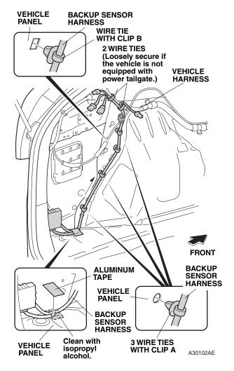
41. Route the backup sensor harness up along the vehicle harness, and secure it to the vehicle panel and vehicle harness with three wire ties with clip A, one wire tie with clip B, and two wire ties. If the vehicle is not equipped with the power tailgate, loosely secure the two wire ties.
