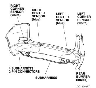
81. Secure the two subharness clips into two center sensor clips.
