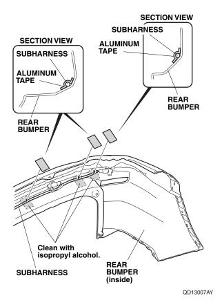
84. Secure the subharness to the rear bumper with three aluminum tapes at the areas shown.
