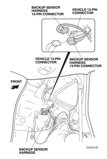
49. Plug the vehicle 13-pin connector into the backup sensor harness 13-pin connector.
