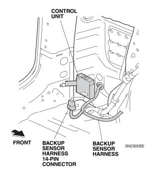
If the vehicle harness is installed in the area shown, continue with step 38; otherwise, go to step 40.
