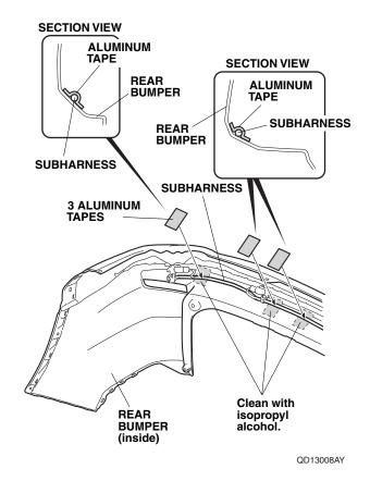
86. Secure the subharness to the rear bumper with three aluminum tapes at the areas shown.
