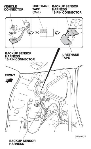
44. Using scissors, cut one urethane tape as shown. Attach the cut piece of urethane tape to the backup sensor harness 13-pin connector.
