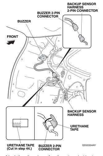
58. Attach the other piece of urethane tape (cut in step 44) around the buzzer 2-pin connector.
