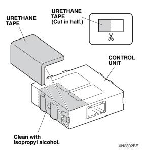
33. Using scissors, cut one urethane tape in half. Attach the cut piece of urethane tape to the control unit in the area shown.
