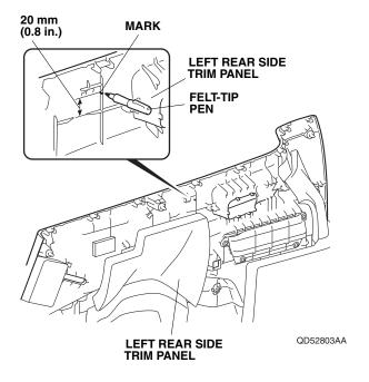
61. Using an utility knife, cut off the ribs on the left rear side trim panel. Remove any burrs.
