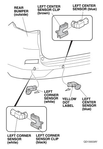
77. Secure the left corner sensor (white) and left center sensor (blue) with left corner sensor clip (black) and left center sensor clip (brown) as shown.
