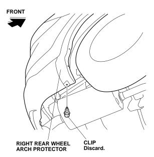
12. Using a pushpin, pierce the center of inner clip on the right rear inner fender.
