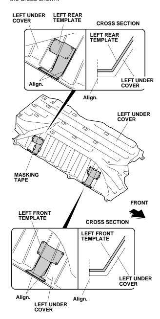
5. Using a pushpin, pierce the six marks on each templates.
