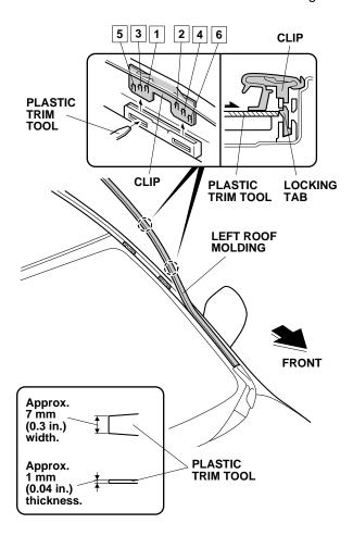
Place a blanket over the roof of vehicle under the left roof molding. Be careful not to deform the roof molding when measuring and cutting.
