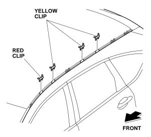
Using a flat-tip screwdriver wrapped with electrical tape, remove the left roof molding cover from the left roof molding (one retaining tab). Discard the left roof molding.
