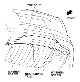
21. Torque the two washer-screws to 0.4 N·m (0.3 lbf·ft).
