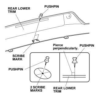
9. While wearing eye protection, drill the two pierced marks to 20 mm. First drill with a 3 mm drill bit, and finish with a 20 mm hole saw.
