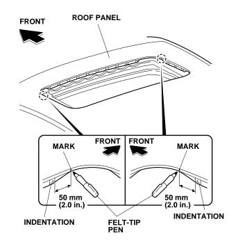
4. Using isopropyl alcohol on a shop towel, clean the roof area where the protective tape will attach. Do not wipe off the mark.
