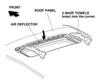
2. Open the moonroof. Roll up two shop towels, and insert them between the roof panel and air deflector to lower the air deflector. Take care not to damage the air deflector.
