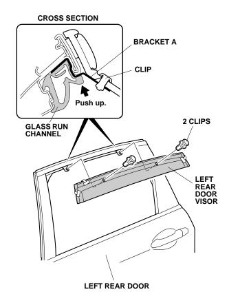
Adjust the end gap of the left rear door visor as shown.
