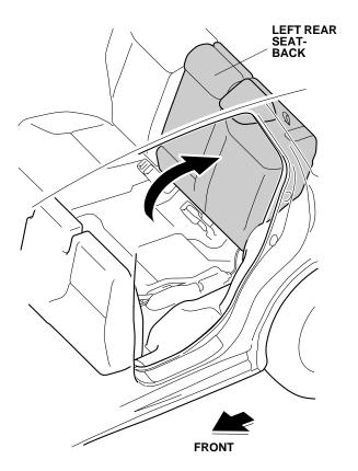
5. Remove the left rear door sill trim (three clips, five retaining tabs, and one hook).
