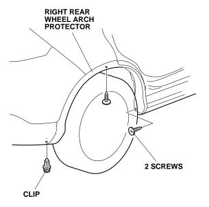
23. Remove the right rear wheel arch protector (eleven clips and two retaining tabs).
