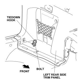
16. Pull away the weatherstrip from the left rear side trim panel at the tailgate opening, and pull away the left rear door opening seal. Starting at the front, release the left rear side trim panel (eight clips and seven retaining tabs).
