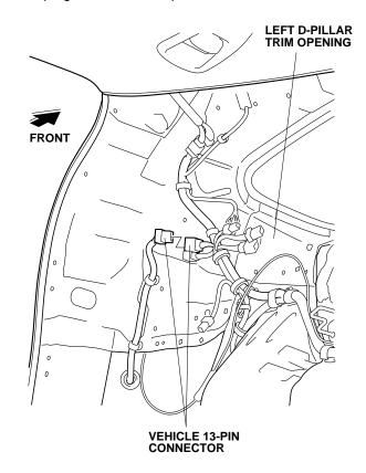
43. Slide the clip on the backup sensor harness 13-pin connector onto the vehicle connector clip.
