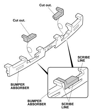
80. Reinstall the bumper absorber to the rear bumper beam.
