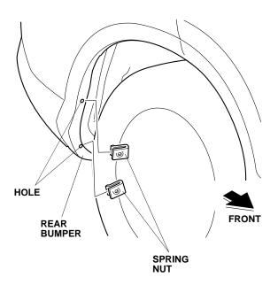
15. Install the right rear splash guard to the rear bumper with three washer-screws in the order 1 → 2 → 3. NOTE: Check there is no gap between the right rear splash guard and the vehicle body. If there is a gap, loosen the three washer-screws, hold the splash guard against the body, and retighten the screws.
