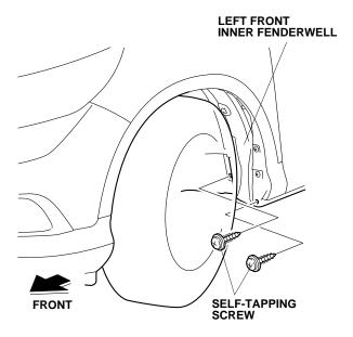
4. Install the left front splash guard to the left front inner fender with one washer-screw and two self-tapping screws removed in step 3 in the order 1→2→3. NOTE: Check there is no gap between the left front splash guard and the vehicle body. If there is a gap, loosen the one washer-screw and two self-tapping screws, hold the splash guard against the body, and retighten the screws.
