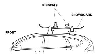
11. If the bindings cannot be positioned between the front and the rear attachments, install the the rear binding behind the rear attachment as shown.
