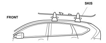
9. If the bindings cannot be positioned between the front and the rear attachments, install the skis with the front bindings behind the rear attachment as shown.
