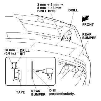
6. Get the rear lower trim. While wearing eye protection, drill the outer holes using a 5 mm drill bit. Remove all burrs.
