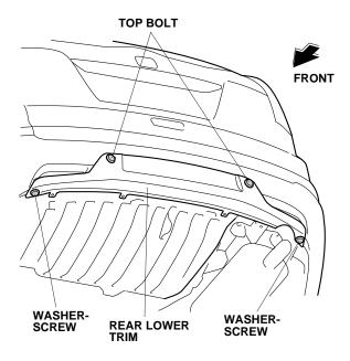
21. Torque the two washer-screws to 0.4 N·m (0.3 lbf·ft).
