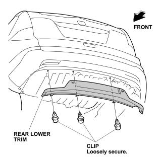
3. Using a pushpin, pierce the rear bumper through the four holes in the rear lower trim, then remove the rear lower trim.
