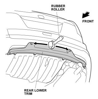
19. Using a rubber roller, apply pressure against the lower portion of the rear lower trim and roll from one end to the other.
