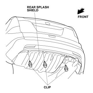
2. Position the rear lower trim on the rear bumper, and loosely secure the rear lower trim with three clips removed in step 1.
