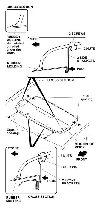
15. Tighten two screws and two nuts on each side of the vehicle first, then tighten two screws and two nuts on the front. Tighten while applying pressure so that there is no gap between the brackets and the roof panel. Torque the screws to 2 N·m (1.5 lbf·ft).
