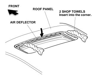
2. Open the moonroof. Roll up two shop towels, and insert them between the roof panel and air deflector to lower the air deflector. Take care not to damage the air deflector.
