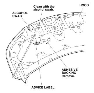
Remove the adhesive backing from the advice label, and attach the advice label to the hood in the area shown.
