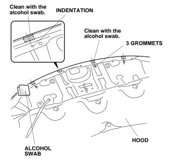
Remove the adhesive backings from each protective film, and attach the four protective films around the front of the hood. Use the three grommets and the indentation as reference. Wrap half of the protective film around the lip of the hood at each of the four locations.
