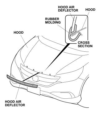
Align the holes in the hood air deflector with the holes in the four brackets. Secure the hood air deflector to the brackets with two screws, two collars, and two clips. Tighten the screws securely.
