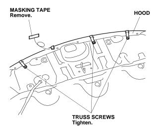
Using an alcohol swab, clean the inside the hood where the advice label will attach.
