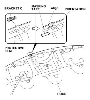
6. Gently close the hood. Position the hood air deflector on the hood and adjust the rubber molding around the front of the hood as shown.
