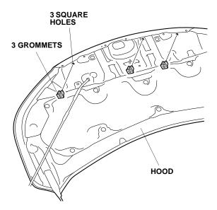
2. Using an alcohol swab, clean the hood where each protective film will attach.
