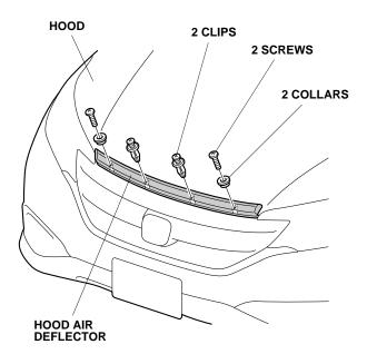
8. Open the hood. Tighten three truss screws loosely installed in step 4. Remove the masking tape attached in step 5.
