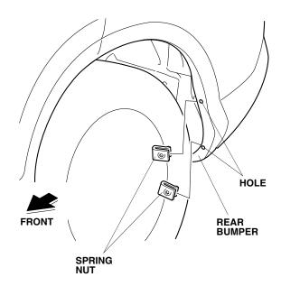
Install the left rear splash guard to the rear bumper with two washer-screws in the order 1→2.
