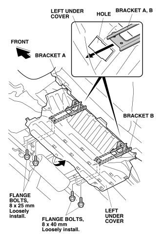
21. With the help of an assistant, bring the left under cover close to the vehicle and loosely install bracket A and bracket B to the vehicle panel using two 8 x 25 mm flange bolts and two 8 x 40 mm flange bolts
