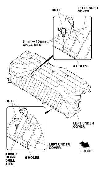
8. Using an air saw, cut out the left under cover in the areas shown. Remove any burrs.
