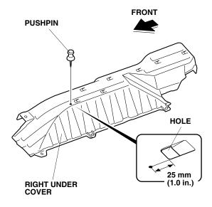
11. While wearing eye protection, drill the pierced mark on the right under cover with a 3 mm drill bit, then enlarge the hole to 10 mm using a 10 mm drill bit.
