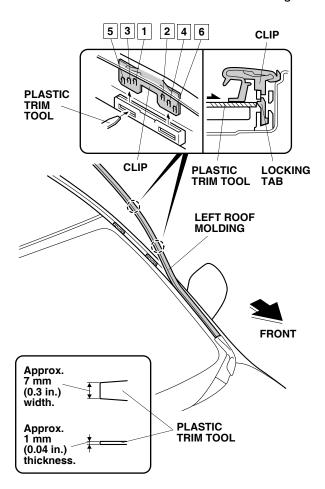
5. Place a blanket over the roof of vehicle under the left roof molding. Be careful not to deform the roof molding when measuring and cutting.
