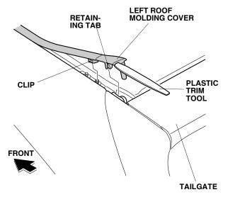
Pull the left roof molding toward the outside of vehicle to release the locking tab, and then press the locking tab toward the inside of vehicle, and release the left roof molding from the vehicle. When removing the left roof molding, start from the rear of vehicle and work towards the front.
