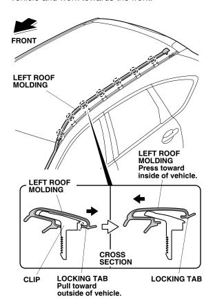
4. While pulling up the left roof molding, remove the two clips. Insert the plastic trim tool alternately to each slots in the clip, and release the locking tabs in the order shown. When removing the left roof molding, start from the rear of vehicle and work towards the front. Be careful not to deform the roof molding.
