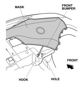
On each side, attach the five plastic hooks to the fenderwell.
