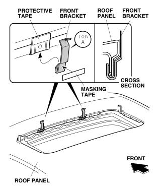
12. Set the moonroof visor on the vehicle roof in front of the moonroof opening, and adjust its position so the holes in the visor are aligned with the holes in the front brackets. Loosely install the moonroof visor to the front brackets with two screws and two nuts. Remove the masking tapes from the front brackets.
