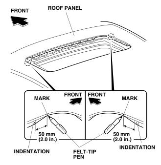
Using isopropyl alcohol on a shop towel, clean the roof area where the protective tape will attach. Do not wipe off the mark.
