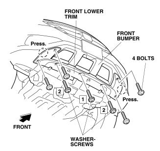
12. Install one bolt into each outboard 13 mm well nut and torque each bolt to 1.0 N·m (0.7 lbf·ft). Press the front lower trim against the front bumper when tightening the bolts on each side.
