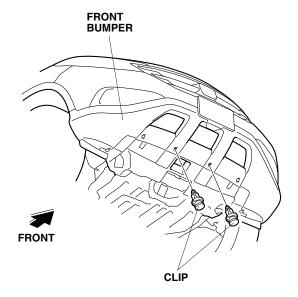
2. Position the front lower trim on the front bumper, and install the front lower trim with the two clips removed in step 1.
