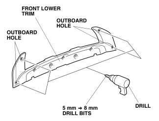
Position the front lower trim on the front bumper, and install it with two new clips. Make sure the rubber molding is not twisted or rolled under the front lower trim.
