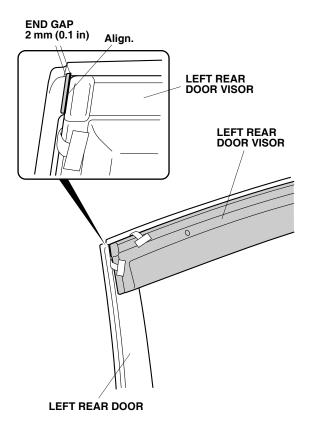
18. While applying light pressure against the left rear door visor, carefully remove the adhesive backings in the order shown. Use your fingers to push up each bracket so there is no gap between the brackets and the door sash.
