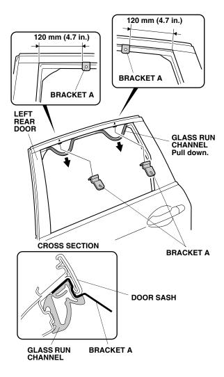
13. Install two brackets A between the door sash and the glass run channel at the measurements shown. Seat the glass run channel properly around the brackets.
