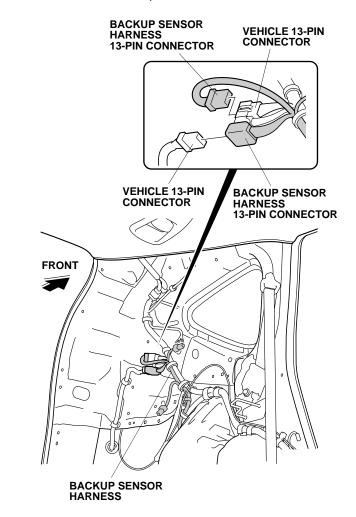
49. Plug the vehicle 13-pin connector into the backup sensor harness 13-pin connector.
