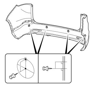
66. While wearing eye protection, drill the eight pierced marks with a 3 mm drill bit. Work from the painted side of the rear bumper. Drill perpendicular to the rear bumper.
