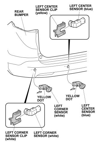
70. Secure the left corner sensor (white) and the left center sensor (blue) with the left corner sensor clip (white) and the left center sensor clip (yellow) as shown.
