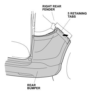
· Release four retaining tabs on each side.
