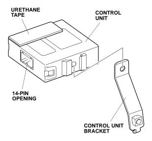
35. Using isopropyl alcohol on a shop towel, thoroughly clean the control unit where the urethane tape will attach. Attach the remaining half of urethane tape (cut in step 33) to the control unit in the area shown.
