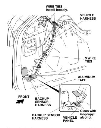
39. Route the backup sensor harness along the vehicle harness. Secure it to the vehicle harness with five loosely-installed wire ties as shown. Go to step 42.
