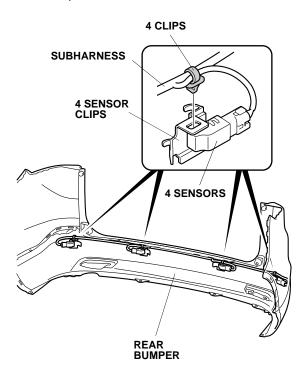
75. On the inside of the rear bumper, use isopropyl alcohol on a shop towel to thoroughly clean the rear bumper where the aluminum tapes will attach.
