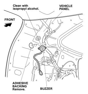
51. Remove the adhesive backing from the buzzer and attach the buzzer to the vehicle panel in the location shown.
