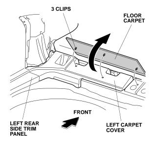
11. Remove the left carpet cover (three clips and two retaining tabs).
