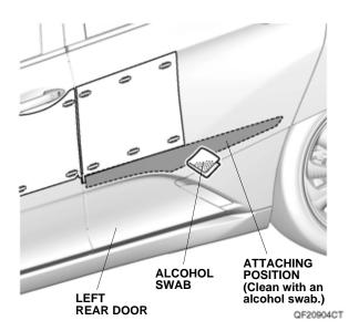
Peel back the adhesive backings, and tape them to the front surface of the left front body side molding with masking tape. Remove the other adhesive backings.
