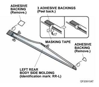
10. Line up the left rear body side molding with the rear template, and install the left rear body side molding on the left rear door.
