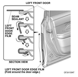
Using a shop towel, wipe the excess 3M protective tape application solution from the left front door edge film. Allow the left front door edge film to thoroughly dry.
