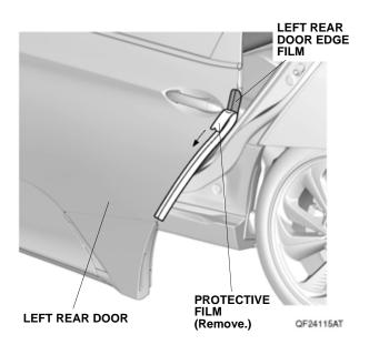
18. Starting from the center and working outward, use your fingers to fold the left rear door edge film around the edge of the left rear door as shown. Move your fingers in one direction only. Attach the left rear door edge film over the seam sealant. Do not trim or damage the seam sealant.
