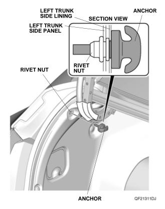
Install three small washers and one bolt into one anchor.
