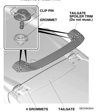
3. Remove the four grommets from the tailgate.
