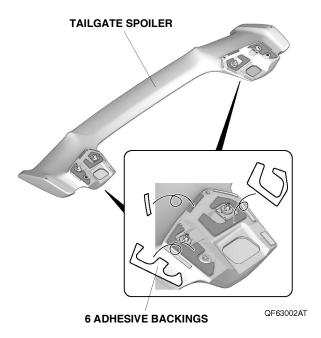
With the help of an assistant, position the tailgate spoiler on the tailgate and loosely install the two bolts.
