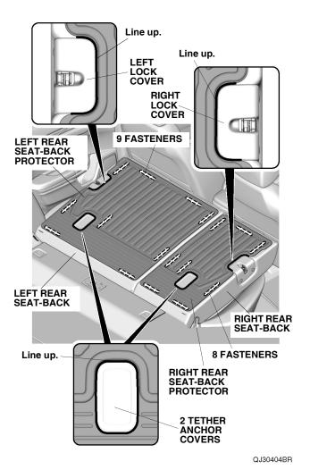
4. Raise and lower the left and right rear seat-backs to confirm the protectors do not interfere with the operation of the seats.
