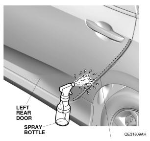
Spray with 3M protective tape application solution.
