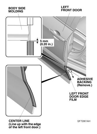
Line up the center line on the lower part of left front door edge film with the edge of the left front door.
