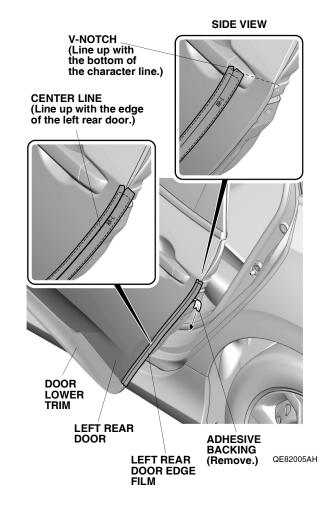
19. Line up the center line on the left rear door edge film with the edge of the left rear door. While applying light pressure, carefully remove the adhesive backing and attach the left rear door edge film to the left rear door.
