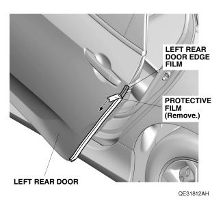
22. Starting from the center and working outward, use your fingers to fold the left rear door edge film around the edge of the left rear door as shown. Move your fingers in one direction only. Attach the left rear door edge film over the seam sealant. Do not trim or damage the seam sealant.
