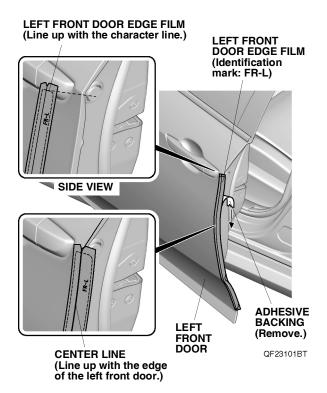
4. Line up the center line on the left front door edge film with the edge of the left front door. While applying light pressure, carefully remove the adhesive backing, and attach the left front door edge film to the left front door. Go to step 10.
