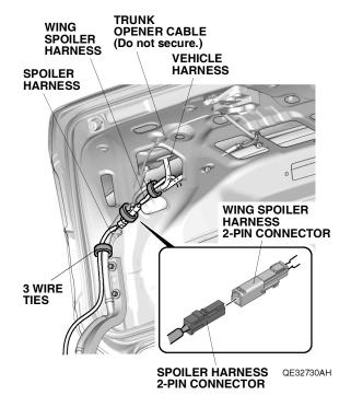
33. Secure the 2-pin connectors, wing spoiler harness, and spoiler harness to the vehicle harness with three wire ties.
