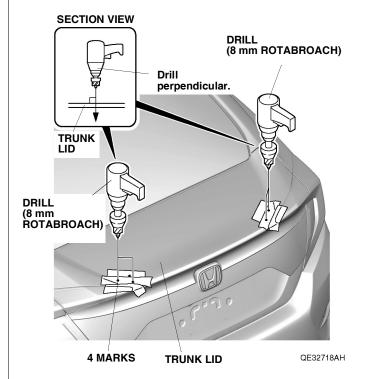
12. While wearing eye protection, use a 10 mm Rotabroach to drill the remaining center-punched mark. Drill perpendicular to the trunk lid.
