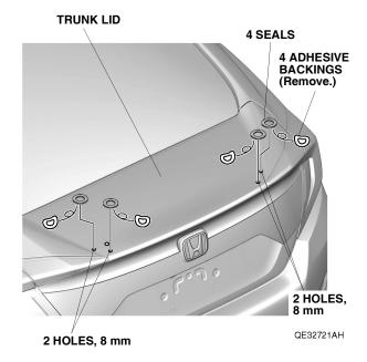
16. Remove the adhesive backings from the other side of the four seals, and route the wing spoiler harness down through the 10 mm hole you just drilled. Seat the grommet in the 10 mm hole.
