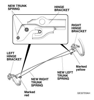
26. Install the center clip to the trunk springs.
