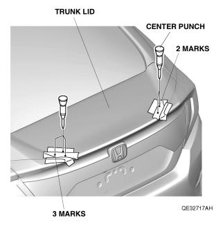
11. While wearing eye protection, use an 8 mm Rotabroach to drill the four outboard center-punched marks. Drill perpendicular to the trunk lid.
