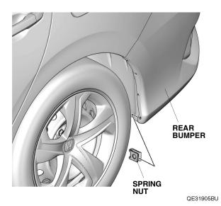
7. Secure the left rear splash guard with two self-tapping screws in the order shown below. NOTE: Make sure there are no gaps between the left rear splash guard and the bumper. If there is a gap, loosen the self-tapping screws, hold the splash guard against the bumper, and retighten the screws.
