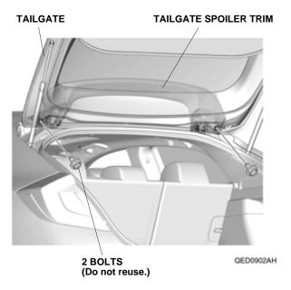
Carefully pull on the tailgate spoiler trim to release the four clip pins from the grommets.
