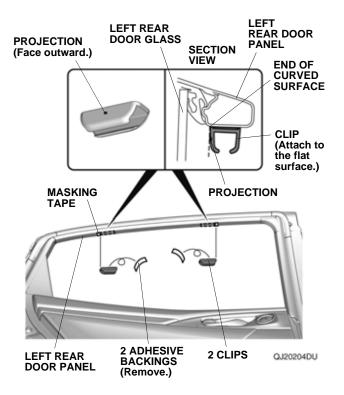
Remove the adhesive backings. Then, line up each clip as shown and attach the clips to the door lining. NOTE: Press down and hold each clip in place for 30 seconds to allow the adhesive to set.
