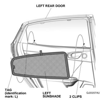
8. Install the top of the left sunshade into the clips, by pulling straight down on the tab.
