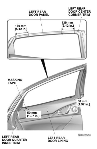
2. Apply masking tape to the left rear door panel and the left rear door lining.
