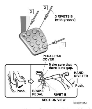
Repeat steps 11 through 14 to install the pedal pad and pedal pad cover on the clutch pedal.
