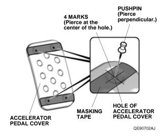
2. Using a pushpin, pierce masking tape as shown.
