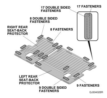
2. Remove the 17 protective clothes from the left and right rear seat-back protectors.
