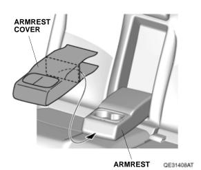
Raise the armrest. Pull out the armrest cover between the armrest and left rear seat-back and secure the fasteners to each other as shown.
