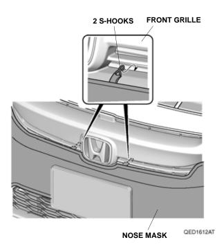
19. Attach the six hooks and two S-hooks to the inside edge of the front lower grille opening as shown.
