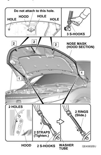
2. Attach the three S-hooks to the underside of the hood by inserting your finger into the belt of each hook.
