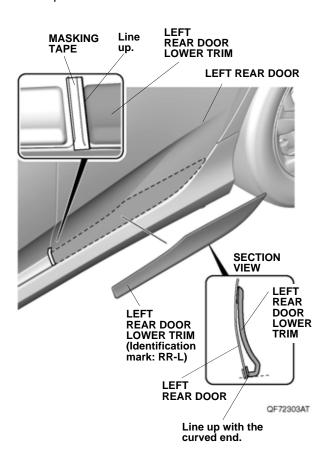
Apply masking tape to the left rear door as shown.
