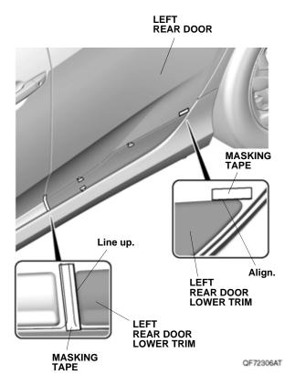
14. While applying light pressure against the left rear door lower trim, carefully remove the taped adhesive backings.
