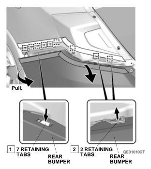
With the help of an assistant, remove the rear bumper. Place the rear bumper on a blanket to prevent damage.
