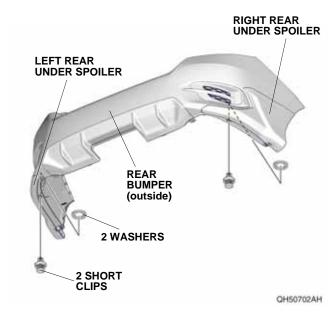
18. With the help of an assistant, install the rear bumper. Then, the left and right rear under spoilers as shown.
