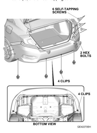
• With center muffler: Remove the two hex bolts, four clips, and six self-tapping screws.
