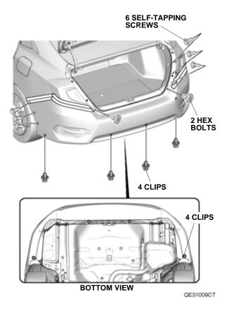
With dual mufflers: Remove the two hex bolts, four clips, and six self-tapping screws.
