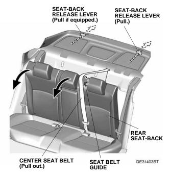
2. Open the trunk. Pull the seat-back release lever, and fold the rear seat-back forward.
