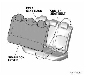
11. Fold down the rear seat-back, and secure the fasteners to each other.
