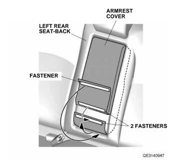
9. Secure the fastener to the left rear seat-back. Go to step 12.
