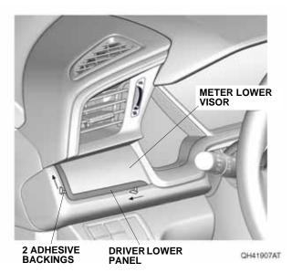
10. Using the palm of your hand, firmly press the driver lower panel against the meter lower visor.
