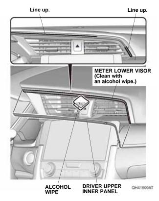
13. Line up the driver upper inner panel with the meter lower visor, and attach it as shown.
