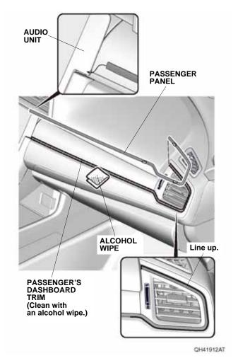
18. Line up the passenger's panel with the passenger's dashboard trim, and attach it as shown.
