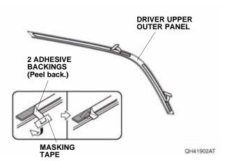
2. Using an alcohol wipe, thoroughly clean the meter lower visor where the driver upper outer panel will attach.
