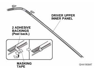
12. Using an alcohol wipe, thoroughly clean the meter lower visor where the driver upper inner panel will attach.
