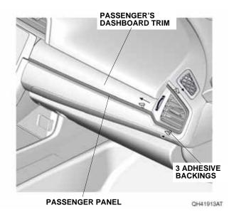
20. Using the palm of your hand, firmly press the passenger panel against the passenger's dashboard trim.
