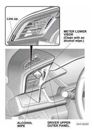
3. Line up the driver upper outer panel with the meter lower visor, and attach it as shown.
