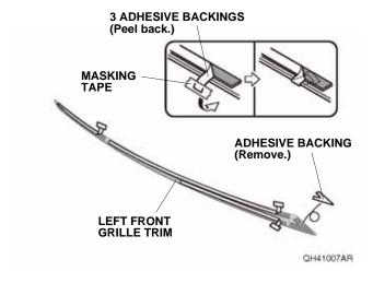
7. Line up the left front grille trim with the left front grille extension, and attach it as shown.
