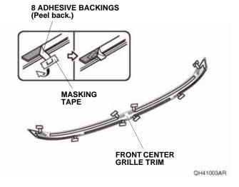
3. Line up the front center grille trim with the front grille, and attach it as shown.
