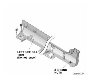
11. Install the three spring nuts on the left spoiler.
