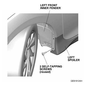
16. Secure the back of the left spoiler with two self-tapping screws.
