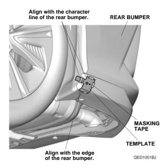
5. Using a felt-tip pen, mark the left rear inner fender along the template.
