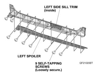
29. Lightly tap the left spoiler to remove any gaps between the left spoiler and the left side sill trim. Tighten the left spoiler with the nine self-tapping screws.
