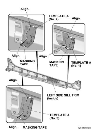
9. Using a pushpin, pierce the center of the mark on each template A.
