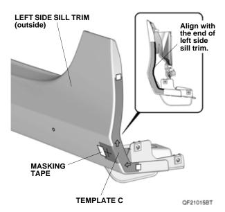
22. Using a pushpin, pierce the center of the mark on template C.
