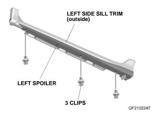
31. Remove the 11 clips from vehicle panel.
