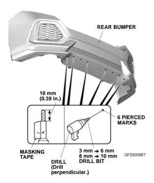
5. Using a file, remove any burrs from the holes.
