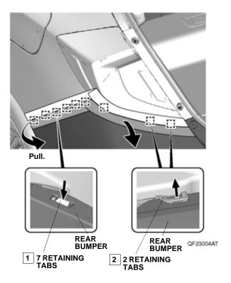
With the help of an assistant, remove the rear bumper. Place the rear bumper on a blanket to prevent damage.
