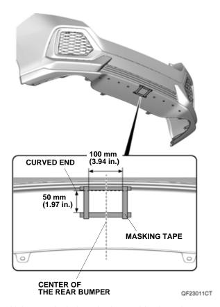
7. Using an alcohol swab, thoroughly clean the rear bumper where the rear under spoiler will attach.
