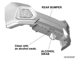
8. Apply the primer to the rear bumper where the rear under spoiler will attach.
