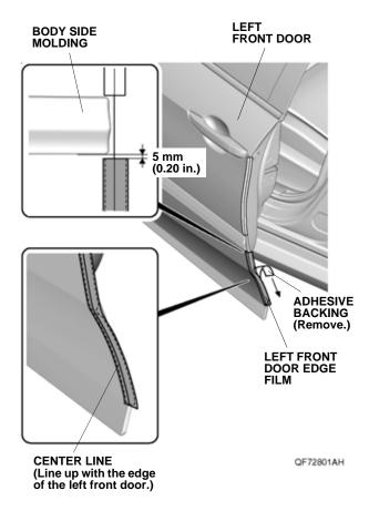
9. Line up the center line on the lower part of left front door edge film with the edge of the left front door. While applying light pressure, carefully remove the adhesive backing and attach the lower part of the left front door edge film to the left front door.
