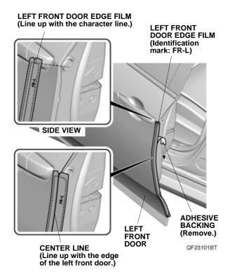
Line up the center line on the left front door edge film with the edge of the left front door. While applying light pressure, carefully remove the adhesive backing, and attach the left front door edge film to the left front door. Go to step 10.
