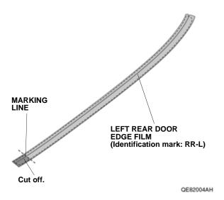
18. Open the left rear door. Peel back about 50 mm (1.97 in.) of adhesive backing from the left rear door edge film. Line up the V-notch with the bottom of the character line on the left rear door as shown.
