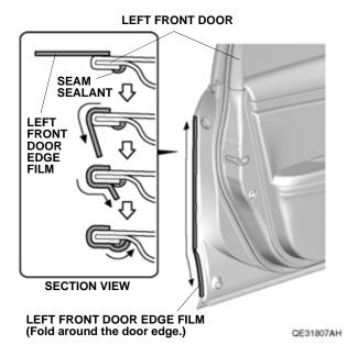
Using a shop towel, wipe the excess 3M protective tape application solution from the left front door edge film. Allow the left front door edge film to dry thoroughly.
