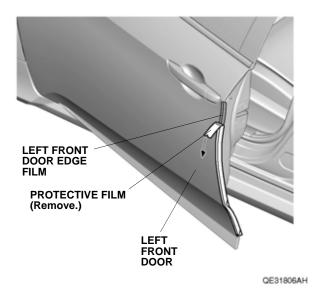
12. Starting from the center and working outward, use your fingers to fold the left front door edge film around the edge of the left front door as shown. Move your fingers in one direction only. Attach the left front door edge film over the seam sealant. Do not trim or damage the seam sealant.
