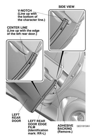
16. Line up the center line on the left rear door edge film with the edge of the left rear door. While applying light pressure, carefully remove the adhesive backing and attach the left rear door edge film to the left rear door. Go to step 20.
