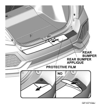
11. Repeat step 8 at the center of the lower section on the rear bumper applique.
