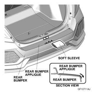
12. Repeat step 9 at the left and right sides of the lower section on the rear bumper applique.
