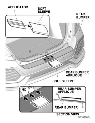
8. Starting from the front and working rearward, use the soft sleeve to smooth out the center of the upper section on the rear bumper applique. Move the soft sleeve in one direction only. If you see an air bubble, stop and gently peel up that section to work out the bubble. Work slowly and keep pressure against the rear bumper applique.
