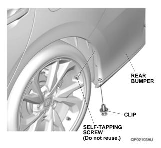
5. Locate the recessed mark. Using a pushpin, pierce the rear bumper at the recessed mark.
